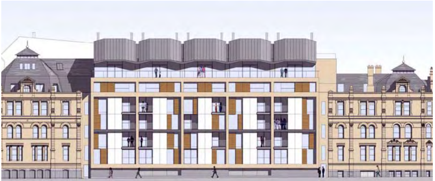
Fig 25a: Coal Exchange, Mount Stuart Square, Cardiff Bay - west elevation. The restoration of the south elevation was a positive outcome of the scheme, though the disabled lift needed to be relocated. The demolition of the west elevation was a considerable price to pay to secure the future of this key building.
