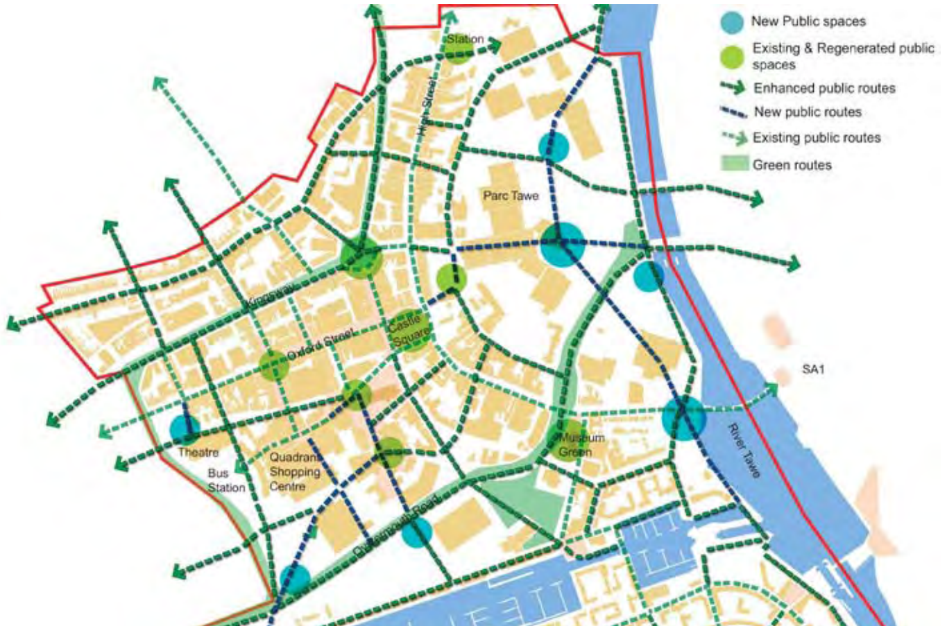
Case Study 1: Swansea City Centre Strategic Framework. The movement and places framework indicated the new pedestrian network and public spaces. The riverside walkway and the new pedestrian link south west from shopping centre to the sea were especially important.
